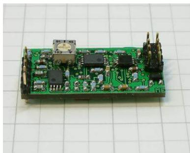
The printed circuit board GSV-3LS contains the most important functions of the GSV-3 series.
