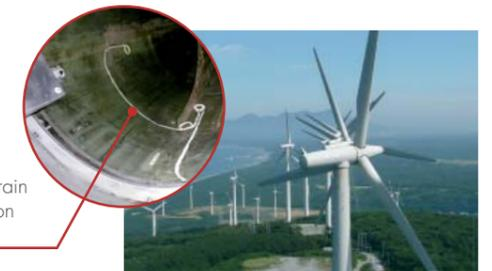
Adhesive bonding of strain & temperature sensors on wind turbine blade
