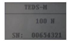
After app. 2 seconds the display will show the measure value (here with a sensor KAM/1kN)
