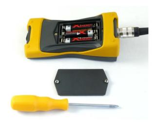
The device will be delivered with batteries mounted. To exchange the batteries open the battery compartment with a Philips screw driver. Remove the batteries if they might not be used for a very long time e.g. than powering by USB only.
