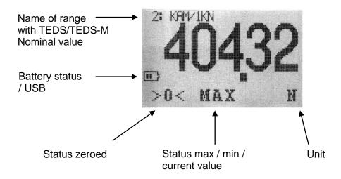
Typical display with masterforce sensor (TEDS-M) connected.
